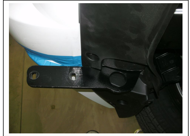
Figure 4: Lower spoiler fitted.
